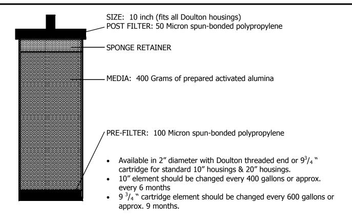
• The A-2 element has also been shown to reduce arsenic to less than 0.02 ppm from 0.12 ppm in the supply water. Total capacity for arsenic has not been determined.
